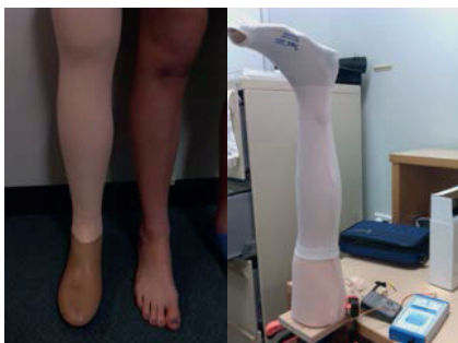
Figure 1: a. The prosthetic limb next to human leg of similar size; b. Prosthetic limb in the testing rig with a compression garment and testing device.
