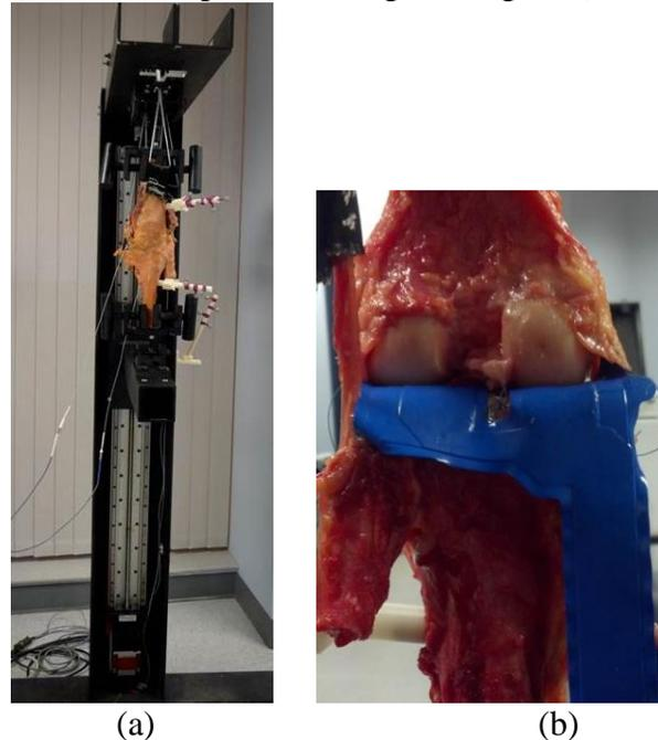
Figure 1. a) knee positioning and loading device and b) posterior view of the knee with sensor inserted.
